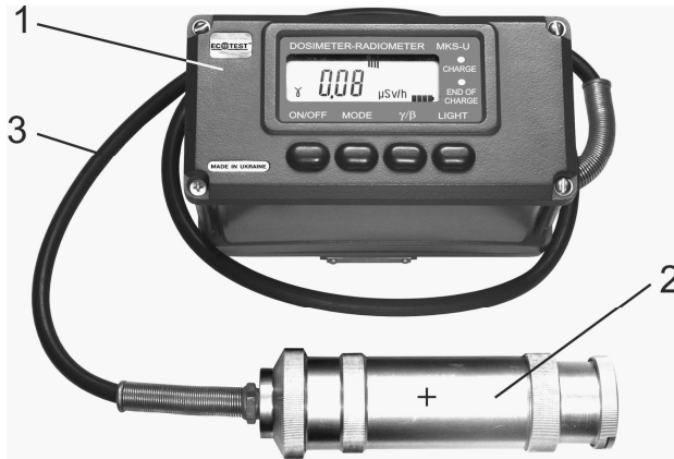
Figure 6 – The control panel of the dosimeter
