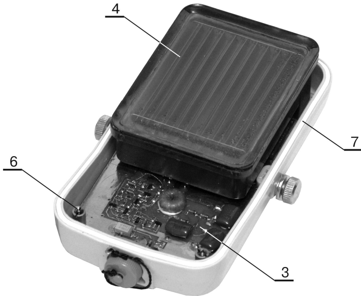
Figure C.3 - BDIB-07 unit with the removed cover
